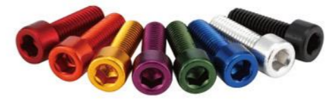
ABC-21408 Spec: AL7075 bolts for bottle cage Size: M5 x 15mm -- 4pcs / set Weight: 4g / set
