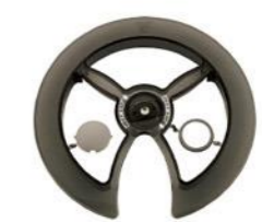
ACC-2602 Spec: PC injection chain guard Crank to chainring distance 6 to 16mm Size: 42 & 44T Weight: 82g --- ditto 46 & 48T Weight: 90g
